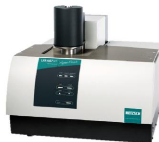
LFA 467 HT HyperFlash ® Suitable for thin samples and high thermal conductivity materials
