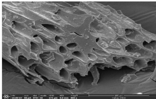
Fig. 1 SEM image of the activated carbon used as the composite substrate (magnitude x800 with 100 \mu\text{m} scale)
