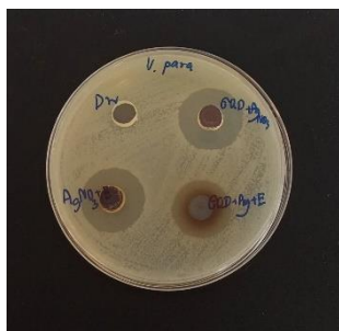
Fig. 3 Zone of Inhibition Area (in mm) exhibited by the formed AgNPs-GQDs against V. parahaemolyticus .
